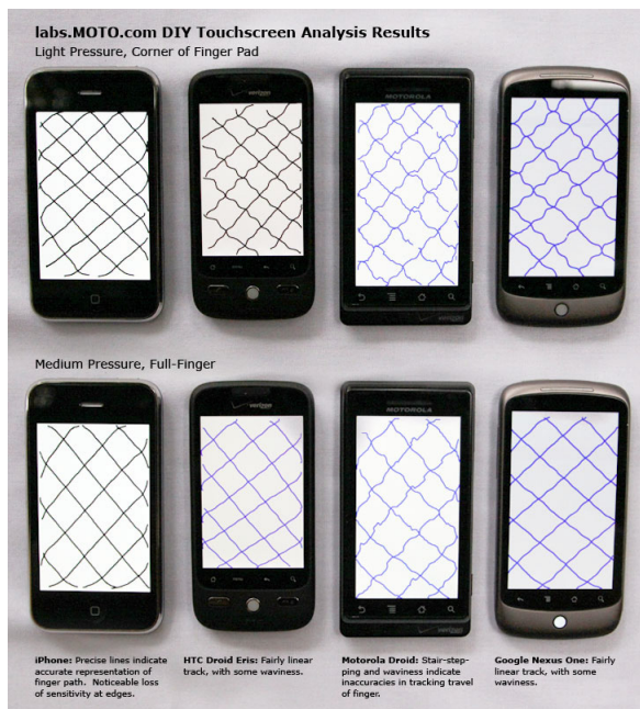
Figure 6 - Linearity of Capacitive Touch Panel by Moto Labs
