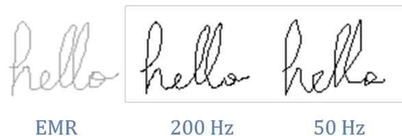
Figure 8- Influence of Scanning Rate on Precision
